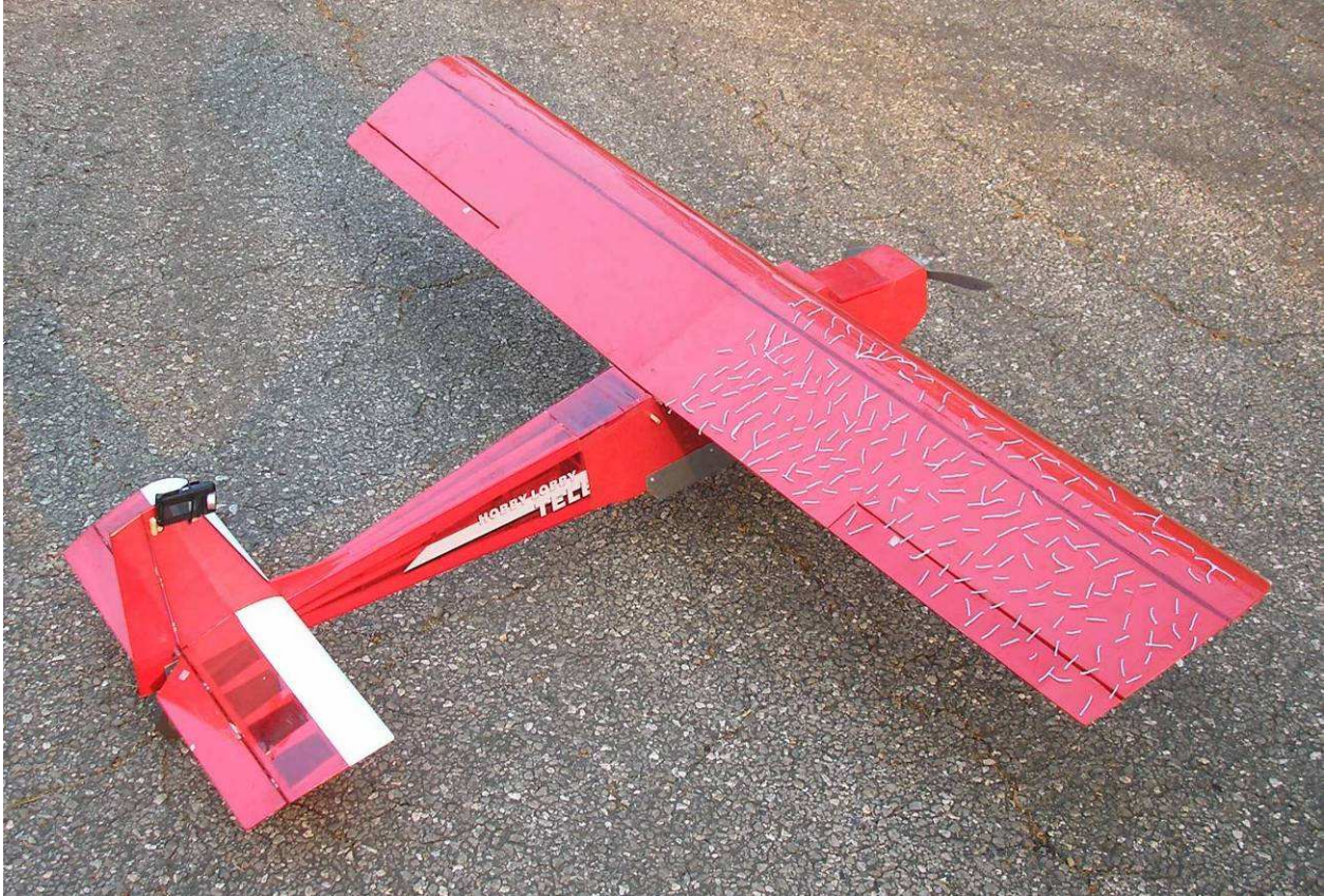
Figure 14: Picture of the final product to be delivered to the sponsor. The microjet arrays cover 100% of the wingspan and can be seen in the darker color red. Tufts, seen on the right wing, will be used to visualize the flow during flight. The video camera, mounted on the tail, is aimed directly at the right wing.
