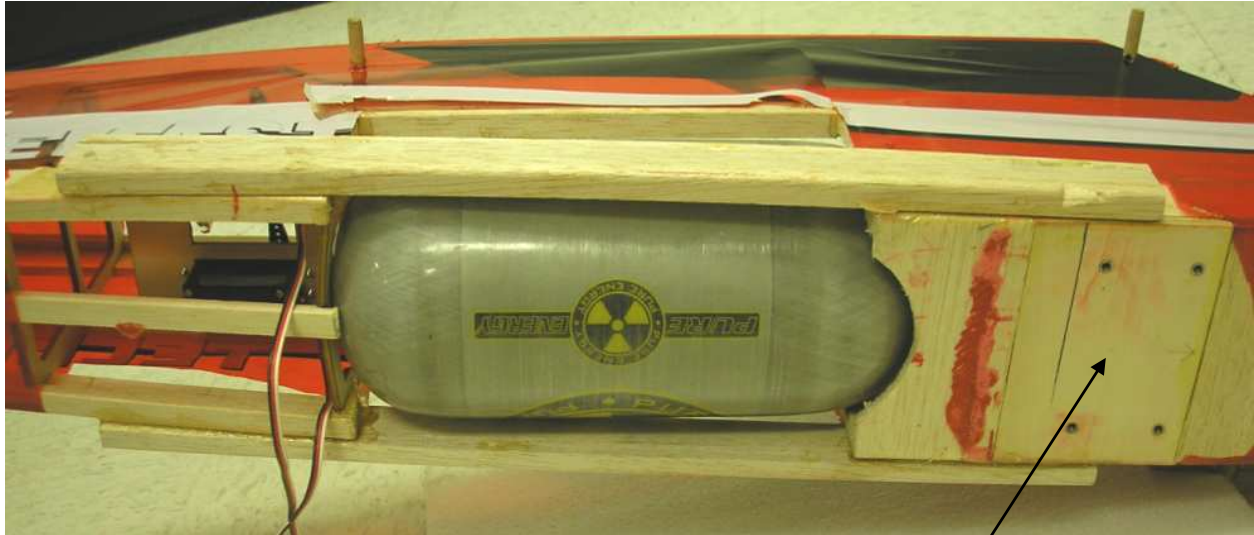
Figure 18: Bottom view of the tank. The location of the landing gear was not modified by its location. A foam support will be installed below the tank as well as a shielding made of sheet metal (Fig. 19).
