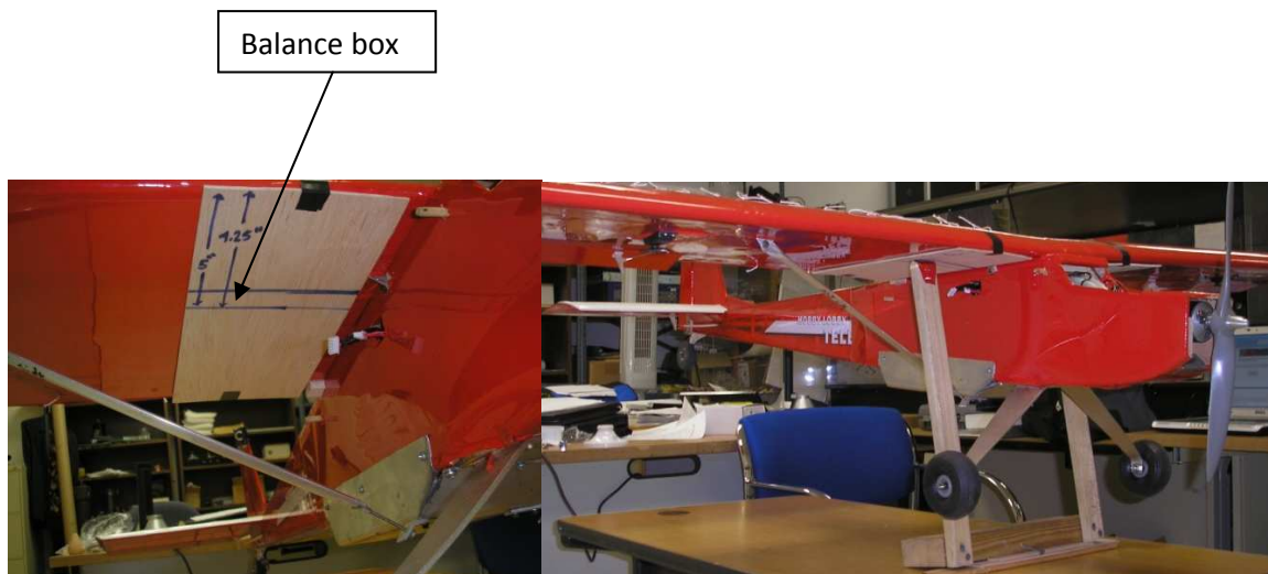
Figure 3, Ensure proper balance by lifting the plane from its wing. Determine the location of level balance. This should reside in the designated balance box.
