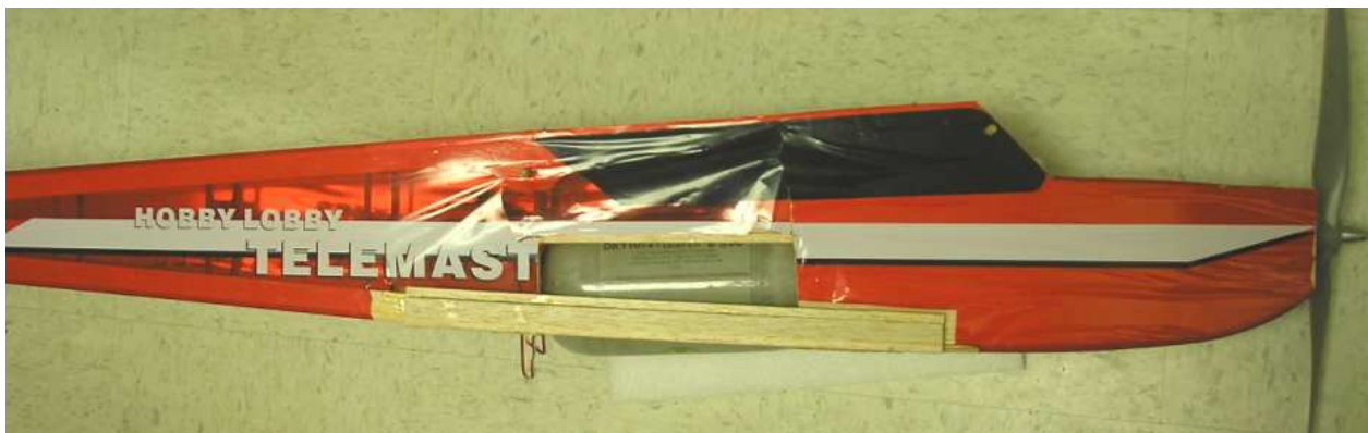
Figure 17: Side view of tank location. As stated, it was recessed in the fuselage. The side of the fuselage is reinforced with an extra wooden support bar.
