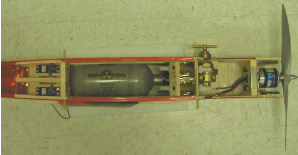
Figure 15: Overhead view of the air supply system placed within the fuselage.
