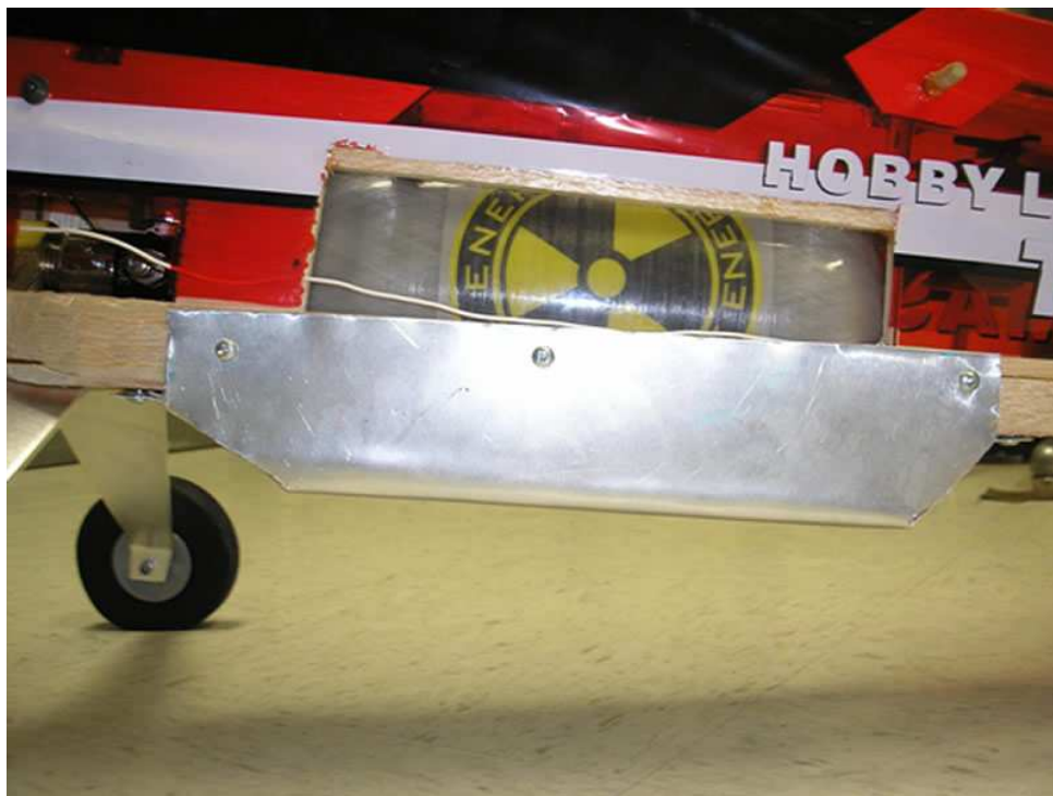
Figure 19: Shielding made of sheet metal (tin) contains the foam support.
